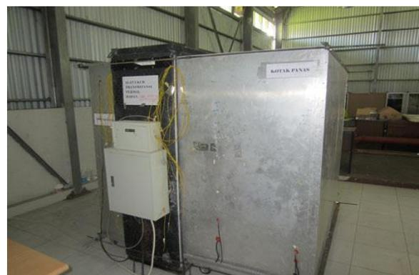
**Figure 3.** Hoxbox in Guarded Laboratory Environment for Getting in-situ Data
