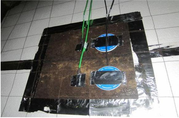
**Figure 4.** Attaching Thermocouples & Heat Flux
