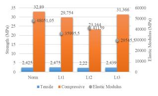
**Figure 7.** Mechanical Properties of Concrete Specimens with Different Fiber Length
