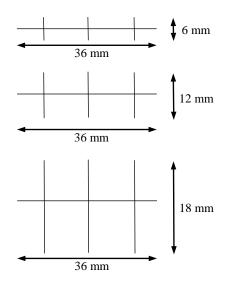
**Figure 3(c).** Geometrical Dimension of PVC Coated Welded Wire Mesh for Different Interlocking Schemes
