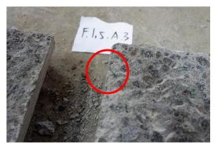
Figure 6. The Full-sized Length of Welded Wire Mesh Sticking Out from the Concrete Surface
