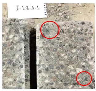
Figure 9. The Uneven Distribution and Irregular Direction of PVC Coated Weld Wire Mesh
