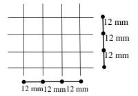
Figure 2. Geometrical Grid of PVC Coated Welded Wire Mesh
