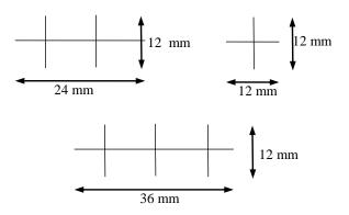
Figure 3(b). Geometrical Dimension of PVC Coated Welded Wire Mesh with Different Length
